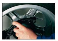
Automatic sensor for measuring the distance of the wheel and for attaching the adhesive weights in the Easy Alu programs. Easy Alu 1, Easy Alu 2 programs are used for balancing alloy rims with maximum precision that need both weights to be attached on the inside.
