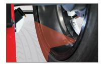
LED spotlight to light up the work area and make it easier to clean the rim, check the wheel and apply weights. The adhesive weights can be positioned extremely rapidly using the laser pointer at 6 o'clock (optional).
