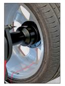
3 Modes to position the adhesive weights: weight holfer clip (optional), 6 o'clock laser indicator (optional), or manually at 12 o'clock.
