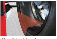
LED spotlight to light up the work area and make it easier to clean the rim, check the wheel and apply weights. The adhesive weights can be positioned extremely rapidly using the laser pointer at 6 o'clock (optional).
