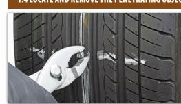
Locate and remove the penetrating object from the tire, noting the direction of penetration.
