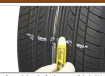
Check tire surface and the valve for the source of the leak(s) by using a leak detector. Mark the injury with a tire crayon.
