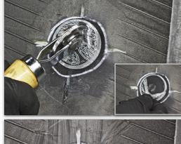
After the repair unit is applied, stitch thoroughly from the center outwards. Always start stitching from the center outward to remove any trapped air that may be under the repair unit. Continue several times in different directions over the whole surface of the repair unit to make sure that it is completely stitched to the innerliner and that it adheres securely to the
