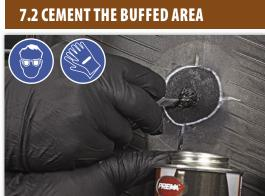
Apply a thin, even coat of PREMA PFC-8 Ultra Fast Dry Vulcanizing Cement to the buffed area of the tire innerliner using a clean brush. Use a swirling motion to apply the cement, as this will aid in the drying process as well as assure a thin, even coat. Completely cover the buffed
