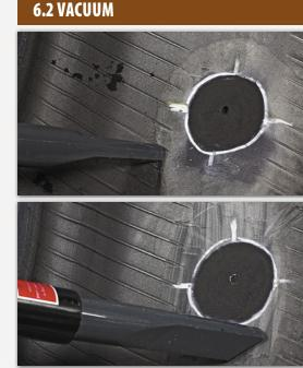
Use a vacuum to remove all debris from the inside of the tire. Do
