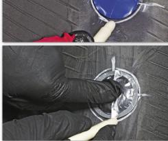
Center the repair unit over the injury and outline an area larger Lightly buff the repair area using a low speed (< 5,000 RPM) air than the unit, so buffing will not remove the crayon marks. If the repair unit has bead arrows, make sure the arrows are
