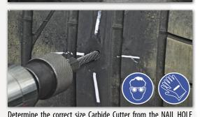
Determine the correct size Carbide Cutter from the NAIL HOLE REPAIR CHART above. Use a low speed tool (not to exceed 1200 rpm) to drill the injury from the inside out two or three times first and then from the outside in once or twice. Use full strokes with the carbide cutter, completely removing the cutter from the tire
