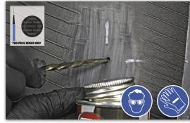
TWO PIECE REPAIR ONLY Apply PREMA PFC-8 Ultra Fast Dry Vulcanizing Cement to the injury channel using a PREMA Spiral Cementing Tool (PSCS).
