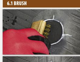
Clean the buffed area with a Brass Brush by brushing the area several times in one direction. Avoid brushing the non-buffed areas where there are contaminants that could be pulled onto the freshly buffed area. Use a brush that is designated only for
