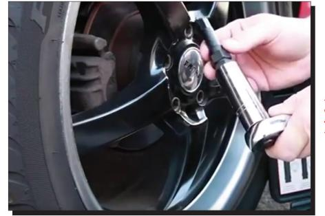
Steelman Locking Lug Master Key Set is designed to remove locking lug nuts on aftermarket vehicles — includes both SAE and Metric sizing.
